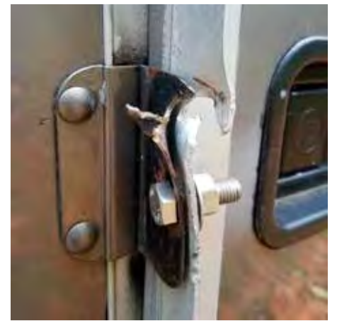
Brute-force damage to Scouts’ storage trailer. Photo: Arne Sewell
