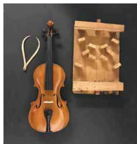
Below: Conscientious objector Howard Scott created the parts for this violin by hand using wood scraps found during his incarceration at McNeil Island during World War II. He also made by hand the calipers and board with pegs, used to bend and shape violin pieces. Violin and tools courtesy the Howard and Ruane Scott family. Image courtesy Washington State Historical Society.
